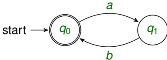
accepts infinite alternating sequences **a b a b ...**
