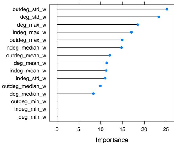
Figure 4: The 15 features of *weighted degree*, the most predictive class, sorted by importance. Note that some of them do not have any contribution to the Kendall- $\tau$  prediction, therefore just few features are necessary in order to estimate the distance.
